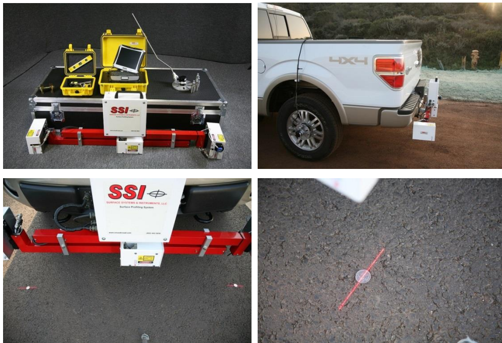
Figure 2-7: Example of a Class I automatic profiler, SSI 9300 Source: (SSI, 2012)
