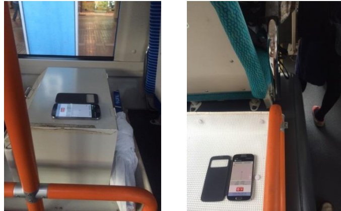
Figure 5-11: Location of the smartphone for IRI Sensing test run
