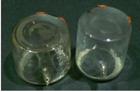
FIG. 10. (Color online) The cells Orvieto, a K-Rb hybrid cell (left), and cell Lottie, a pure Rb cell (right). Despite being in the beam for over ten times as long, cell Orvieto only shows traces of a white film in an area of the cell where a blockage of hot air flow by the cell mount may have caused a cold spot on the cell. Cell Lottie, the pure Rb cell, shows a relatively uniform white film over its surface.
