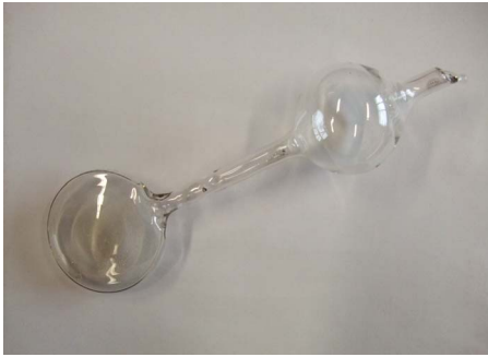
FIG. 12. (Color online) The two chambered cell named “Roadrunner” created several years ago at NIST. The ^3\text{He} spin-relaxation time was 220 h in the laboratory and 135 h in the in situ apparatus installed on the thermal high-flux neutron test beam. This cell was designed for an optical pumping axis parallel to the neutron beam whereas our magnetic cavities are for perpendicular neutron and optical pumping axes. Thus, the stem on the optical pumping volume (right) is not optimal for our conditions because the optical pumping light must pass through this stem which blocks and distorts the collimated optical pumping beam.
