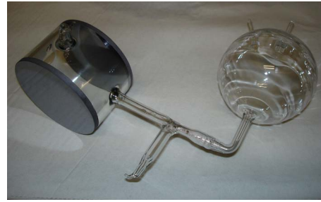
FIG. 11. (Color online) The two chambered cell named “Gemini” created for tests. The optical pumping portion is made of blown GE180 glass and the NSF portion is a Pyrex body with Si windows. The ^3\text{He} spin-relaxation time was 200 h with a 2 h ^3\text{He} polarization transfer time between the chambers.
