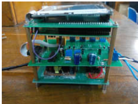
Figure 2. Harmonic distortion analysis prototype
