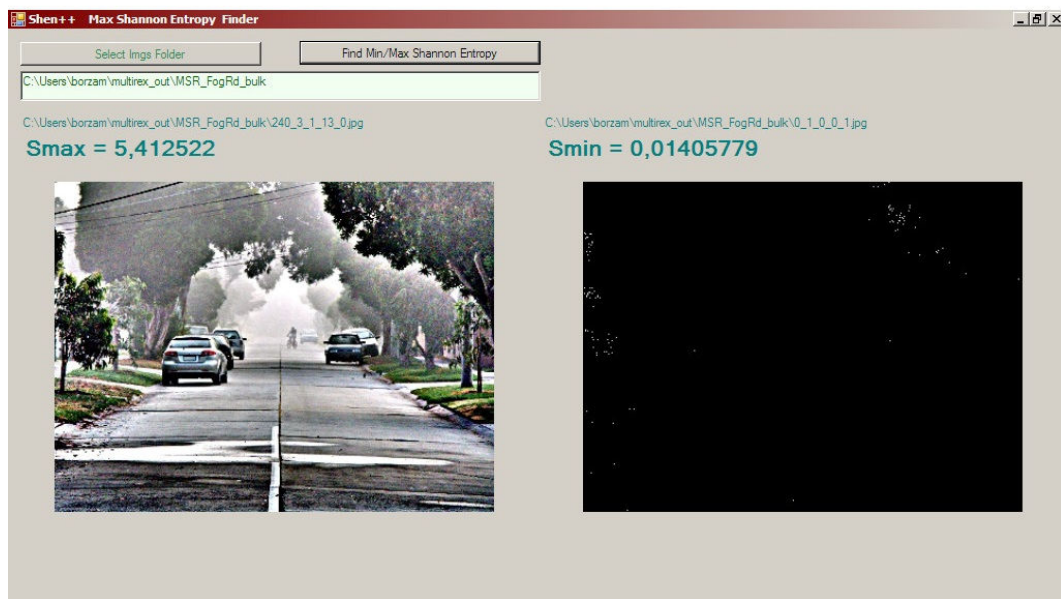
Figure 5: To find the images having the largest and the smallest entropy in a bulk set we have developed the Shen++ Max Shannon Entropy Finder , working on the histogram of the equivalent colour tones. Here we can see the snapshots of two cases. In the upper part, we see the evaluation of entropy on the single, original colour image, from which the grey tone image of Figure 1 had been obtained. Note that, since we have just one image, the maximum and minimum of entropy are coincident. In the lower part, we can see the images having the maximum and minimum of entropy from the bulk set of images generated with GIMP Retinex. The values of the corresponding parameters are encoded in the name of the output image.
