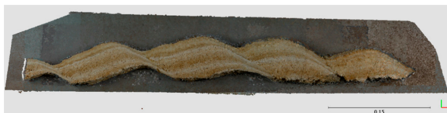
Figure 5. The colored 3D dense point cloud of the rock sample.
