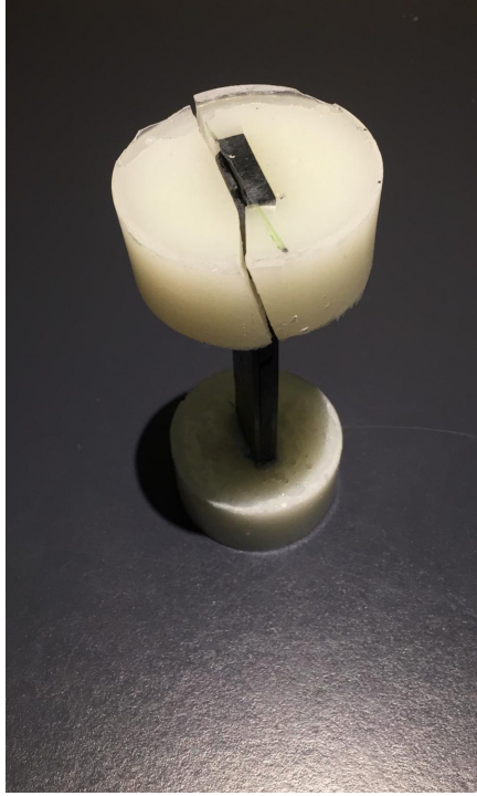
(a) Broken specimen after the buckling test.
