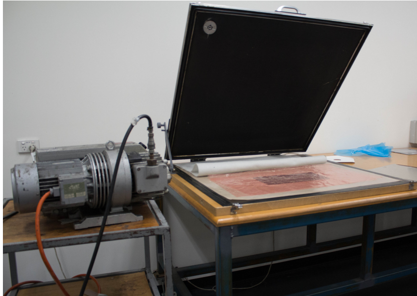
Figure 5.2: Debulking of a CFRP lay-up.
