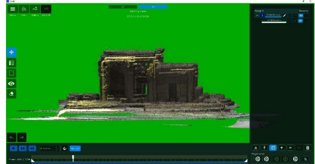
Figure 5. Misalignments between point cloud frames are visible after the acquisition, in yellow a single point cloud frame is highlighted
