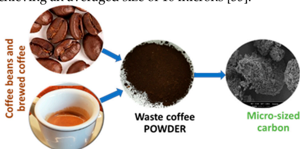
Figure 1. Extraction and conversion of waste coffee powder to carbonized biochar (BC).
