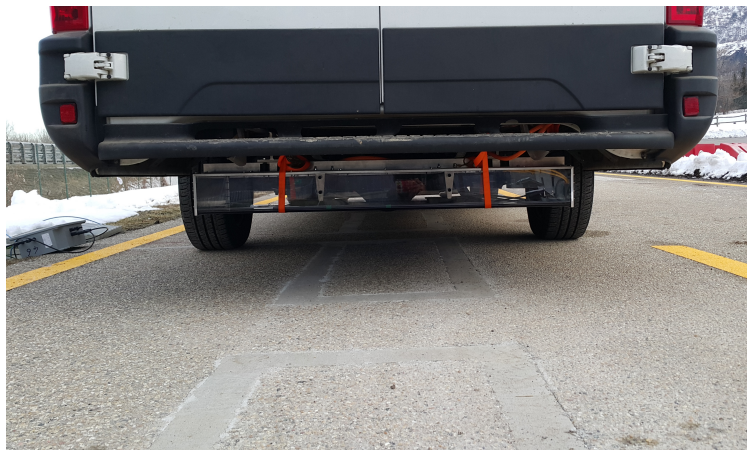
Fig. 5.16: Picture of the receiver structure mounted under the vehicle
