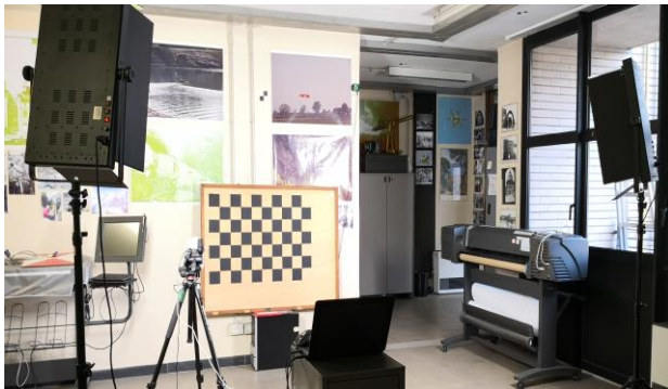
Figure 1. The acquisition of a dataset in indoor environment, considering controlled illumination and exposure values (T2)
