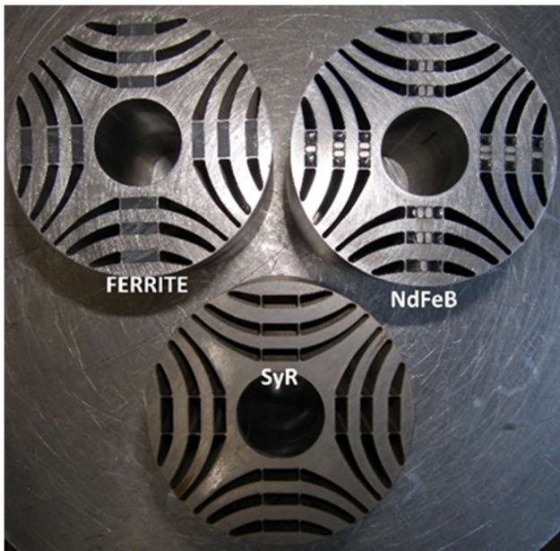
Fig. 5. Picture of the three prototype rotors assembled.
