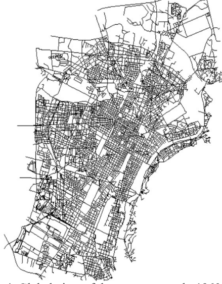
Figure 4. Global view of the water network: 19604 pipes.
