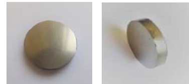
Fig. 2. Sintered Ti 2 AlN MAX phases samples
