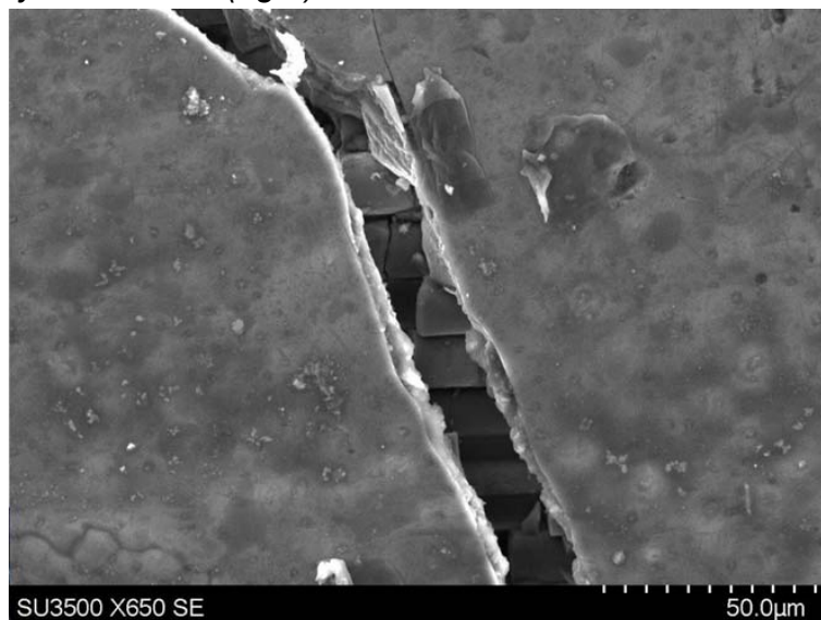
Fig. 10. Sub-surface fibres exposed under in-situ loaded SEM inspection.
