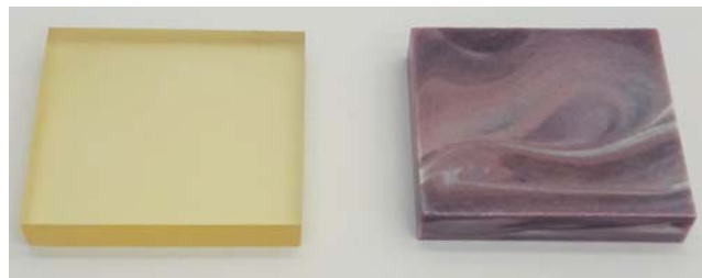
Fig. 2. Fresnoite glass (left) and glass-ceramic (right)
