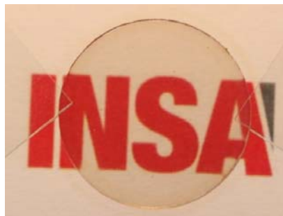
Fig. 4. Spinel sample RIT = 85% at 500 nm for 1.85 mm thickness
