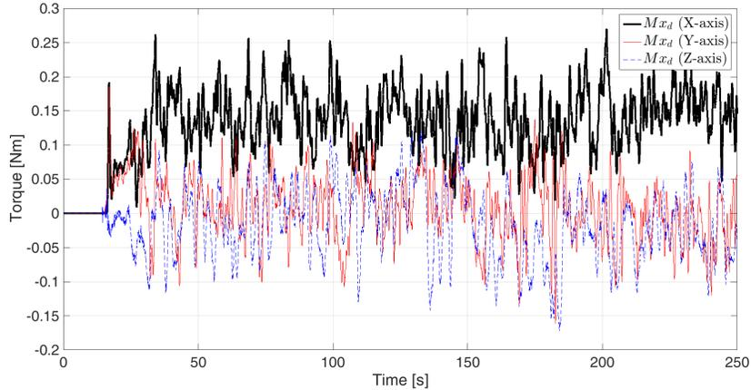
Figure 9: Attitude estimated disturbance: hovering flight test.
