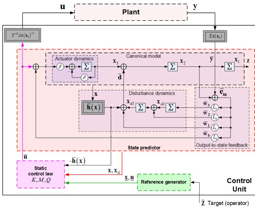
Figure 1: UAV quadrotor attitude digital control unit.
