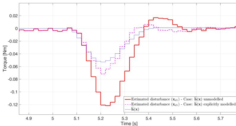
Figure 6: Disturbance estimation: simulation test.
