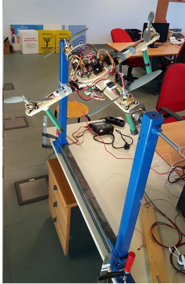
Figure 3: Experimental mono-axial test-bench for multirotor UAVs.
