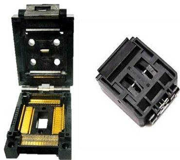
Fig. 2.29 The 160 pins MQFP socket open (left) and close (right). A mechanical pressure of the top cover, guarantee the electrical contact between the ASIC pins and the socket ones.
