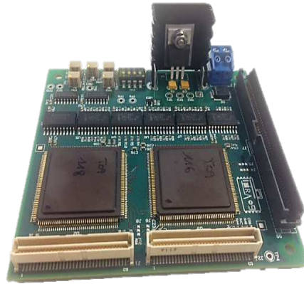
Fig. 2.58 The TERA09 front-end board hosting two ASICs is going to be the new monitor chamber readout electronics, adopted by DETECTOR Devices and Technology Torino.
