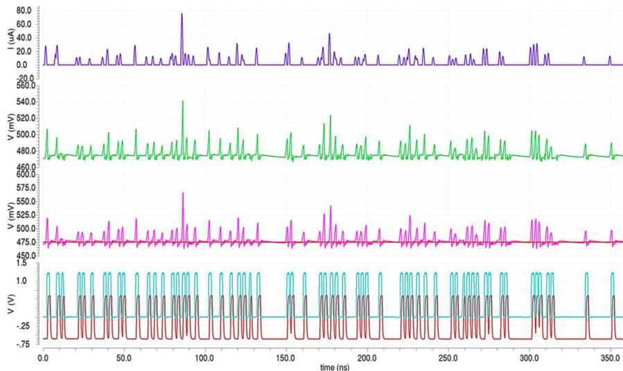
Fig. 3.87 Schematic simulation waveforms for 250 MeV protons at 250 MHz. From the top: the CSA output voltage, the OTA buffer output voltage with the discriminator threshold superimposed, the discriminator output the input signal.
