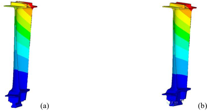
Figure 5.32: deformation of the blade: a) mode shape, b) flutter deformation
