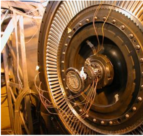
Figure 6.3: test article bladed disk
