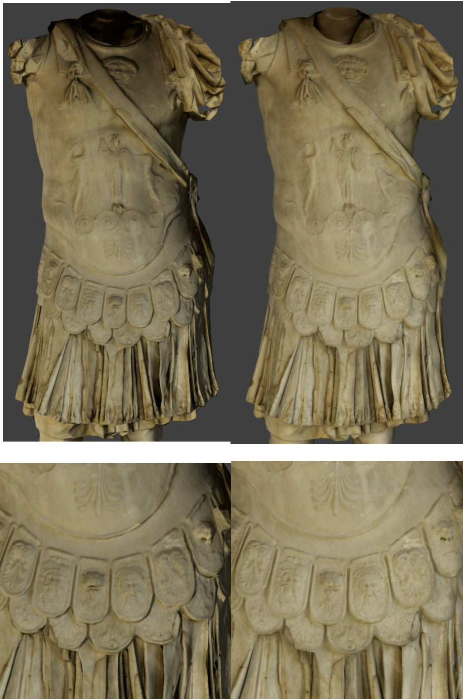
Figure 103. LP with diffuse color and Normal Map(left) and LP with just diffuse color (right).
