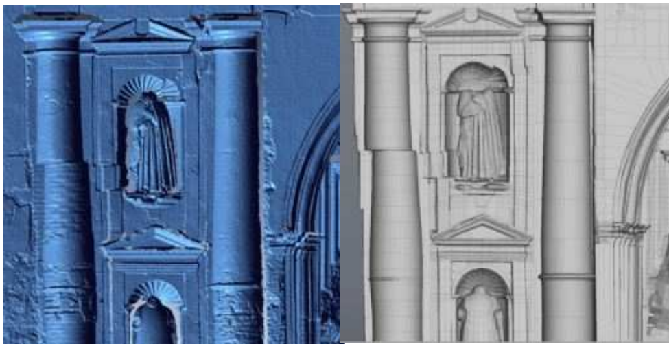
Figure 43. Left: High Poly model; right: corresponding Low Poly model from retopology realized with software Luxology Modo
