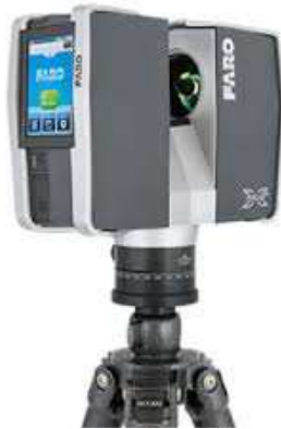
Figure 11. The 3D scanner Faro Focus 3D. A phase shift laser which can be used for projects at architectural scale (1:100-1:50 - Range 0.60-330 m - Accuracy of point position 2 mm at 25 m.
