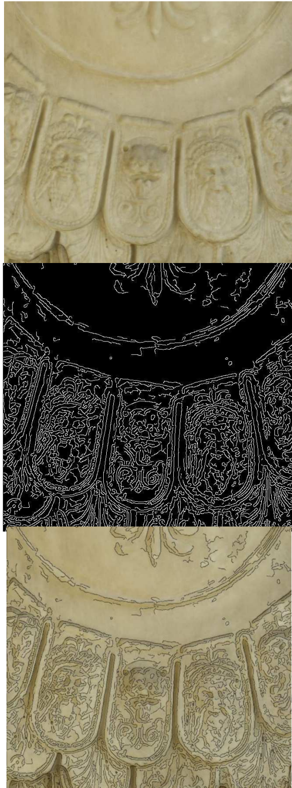
Figure 131. Canny filter HP. Threshold [0.03 0.08] sigma (0.8).
