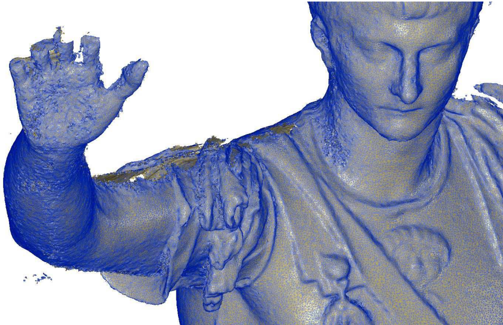
Figure 86. Zoom on the Photoscan mesh in wireframe mode in which the topological errors and the noise are visible.
