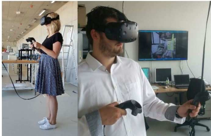
Figure 10. The virtual reality system HTC Vive in use ( www.vive.com ). The screen in the background shows the same sequence as appears to the user in the VR glasses (right). Source: (T P Kersten et al., 2017)
