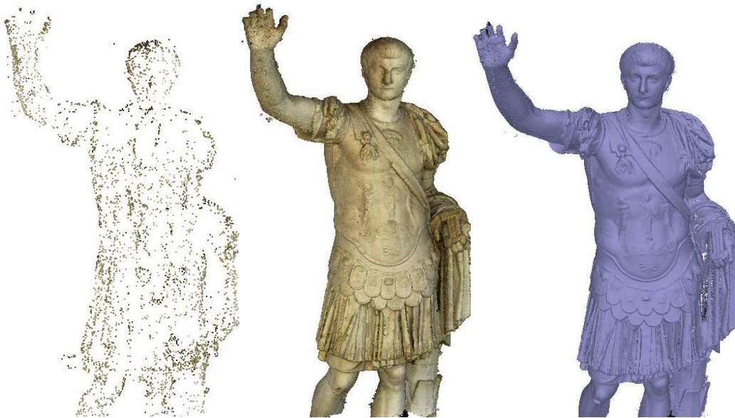
Figure 55. The sparse cloud with tie points extracted, the dense cloud and the final 3D model viewed as smoothed mesh
