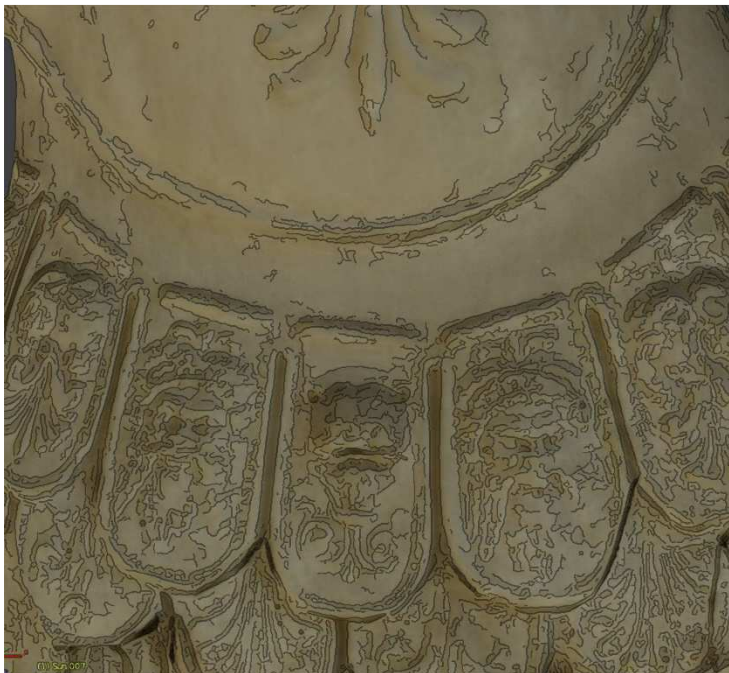
Figure 132. Canny filter - LP model with NM applied. Threshold [0.03 0.08] sigma (0.8).
