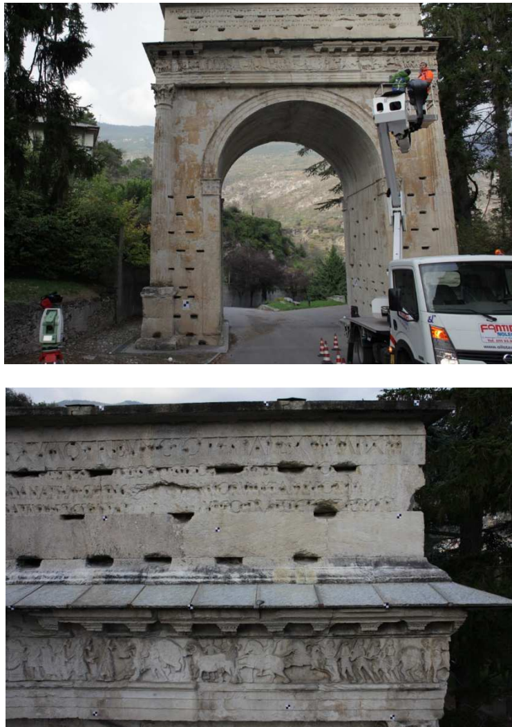
Figure 59. Above: the acquisition step; below: the targets placed on the surface have been measured by a total station and referred to a global reference system.
