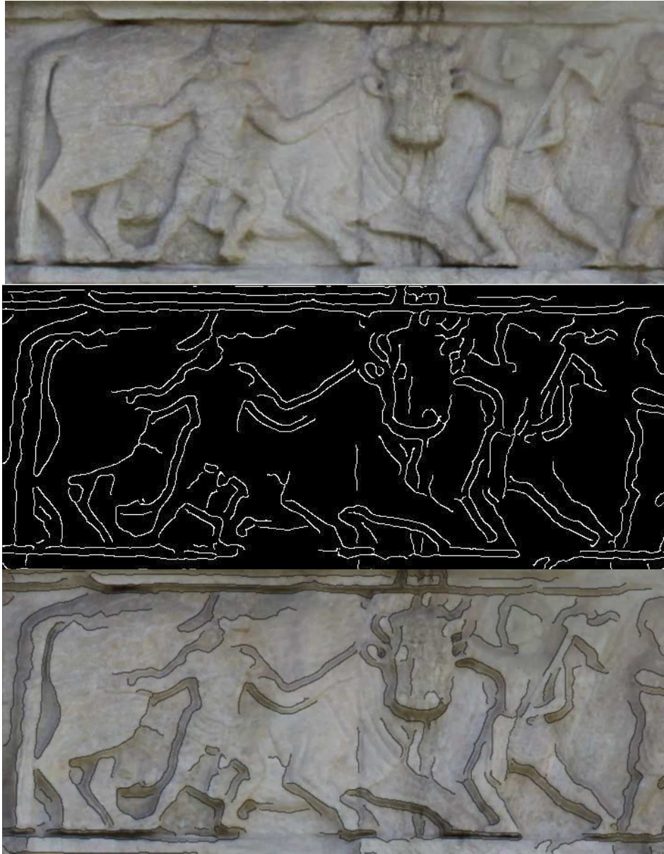
Figure 135. Canny edge detector applied on a zoomed portion of the frieze – HP model- Threshold 0.2, sigma 3.
