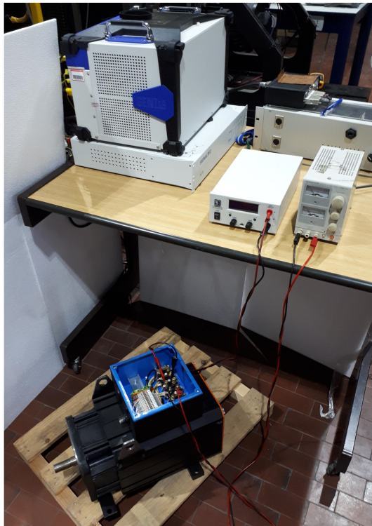
Fig. 9. Experimental setup: dual winding machine, DC power supplies and HBM Gen7i data logger.
