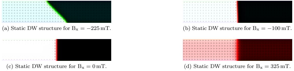
Figure 3.13: Snapshots of DW static structure determined by micromagnetic simulations under longitudinal fields.
