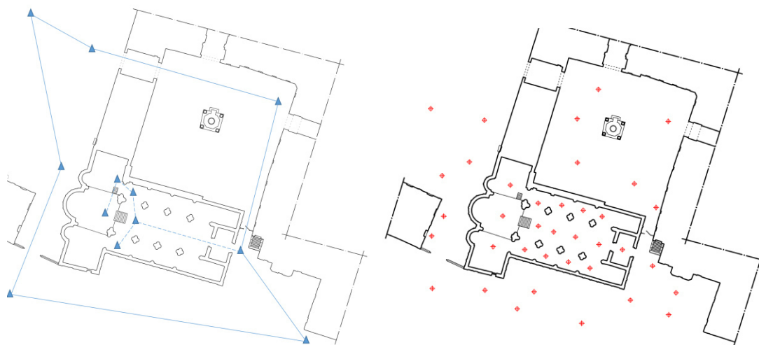
Fig. 1 – The control network (left) and the Laser Scanner station points (right)
