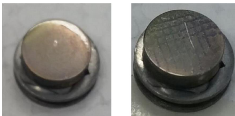
Figure 3.40: Aspect of the sample CT_Mentha oil_water washed before and after making the incisions.
