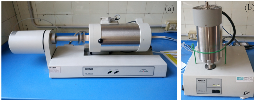
Fig. 3.1 (a) the DIL 404-PC facility used for thermal expansion experiments, (b) the DTA 404-PC used for calorimetry experiments.
