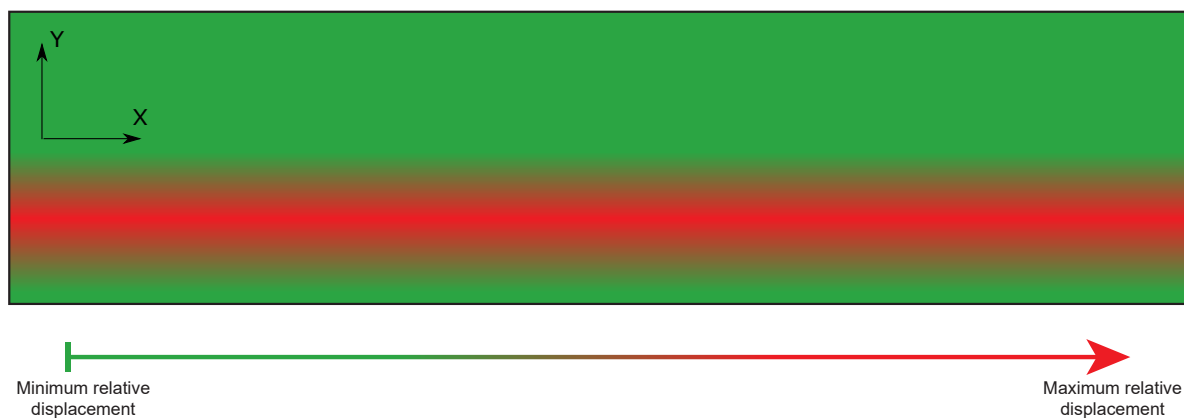
Figure 7. Top blade-strip contact patch view: high mobility region (red) with the largest relative displacement.
