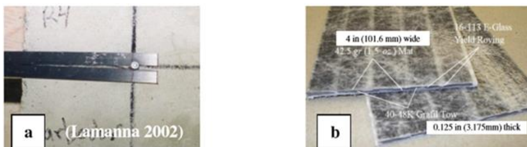
Figure 22: a) splitting failure for EB-FRP laminates; b) laminates used for MF-FRP systems. Source (Ascione, et al., 2009).
