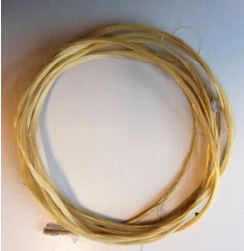
Figure 78: damaged Kevlar® 29 sample (2040 hours)
