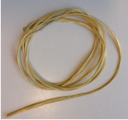
Figure 75: damaged Kevlar® 29 sample (1272 hours)
