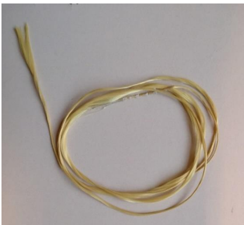
Figure 72: damaged Kevlar® 29 sample (792 hours)
