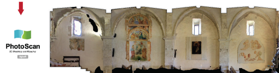
5 3D mesh model created - Retrieving the elevations and sections with Agisoft Photoscan software
