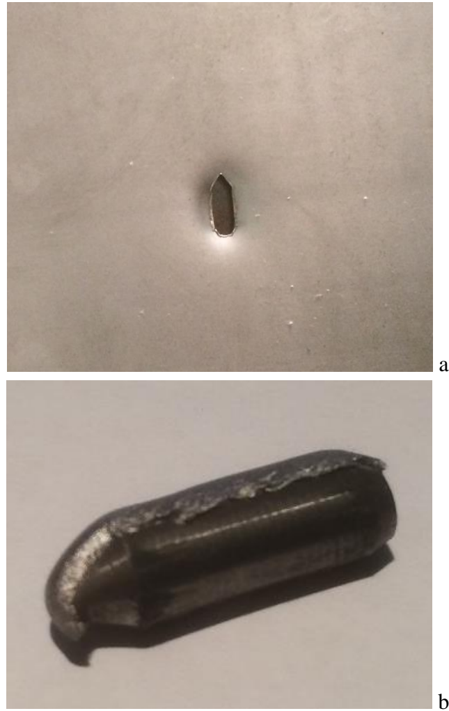
Figure 38: Penetrator pierce the plate with a lateral impact
