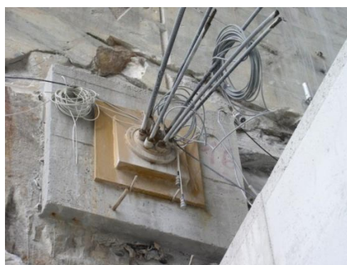
Figure 3. Instrumented tendon head on the left wall of the cavern: an anular load cell at the tendons head with a tiltmeter.
