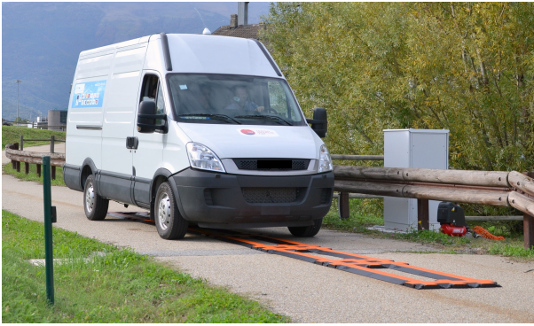
Fig. 10: First prototype of a dynamic IPT system for a light commercial vehicle within the eCo-FEV project (Italy).
