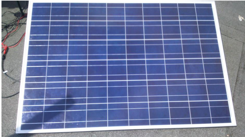
Fig. 15 PV module under partial shade.
