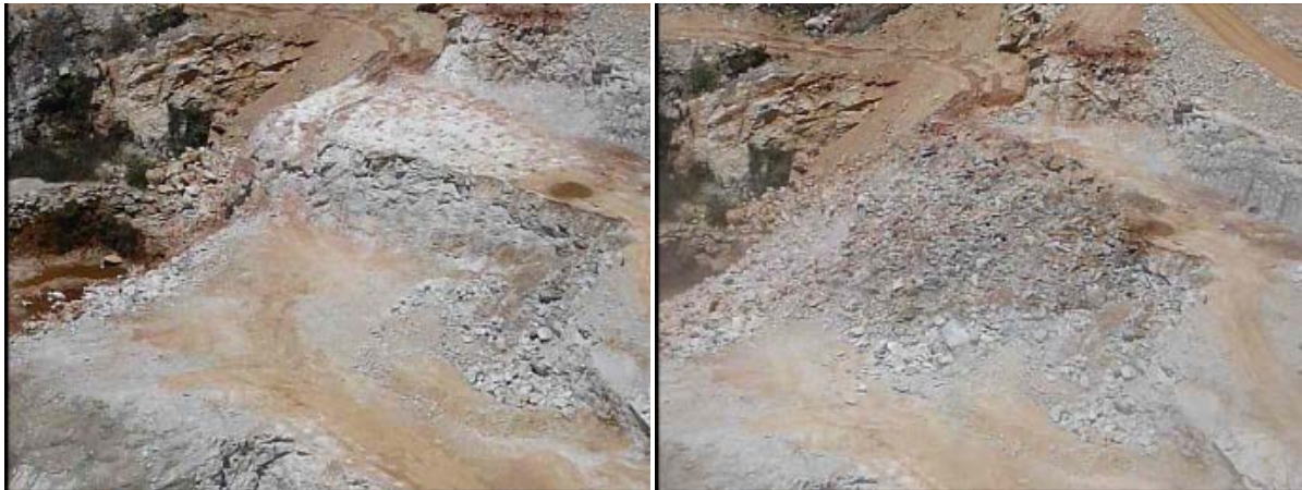
Figure 5. General view of the bench before (left) and after (right) the blast. The free surface, being left by the previous blast, dimensioned according to the proposed method, is smooth and slightly damaged. The muck-pile generated by the blast has a suitable geometry.
