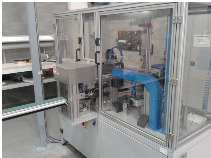
Figure 1.14: Automatic welding process for Si cells.
