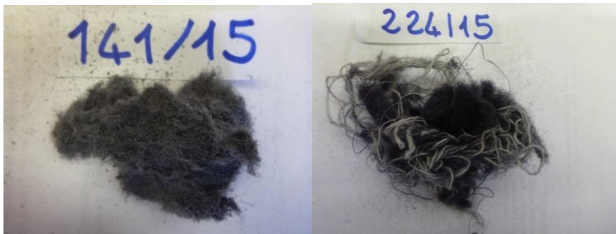
Figure 49: Ambiance (141/15) and machinery sampling (224/15) from twisting process.
