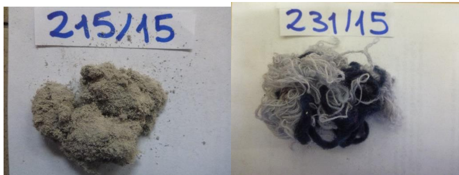
Figure 52: Ambiance (215/15) and machinery sampling (231/15) from winding section.
