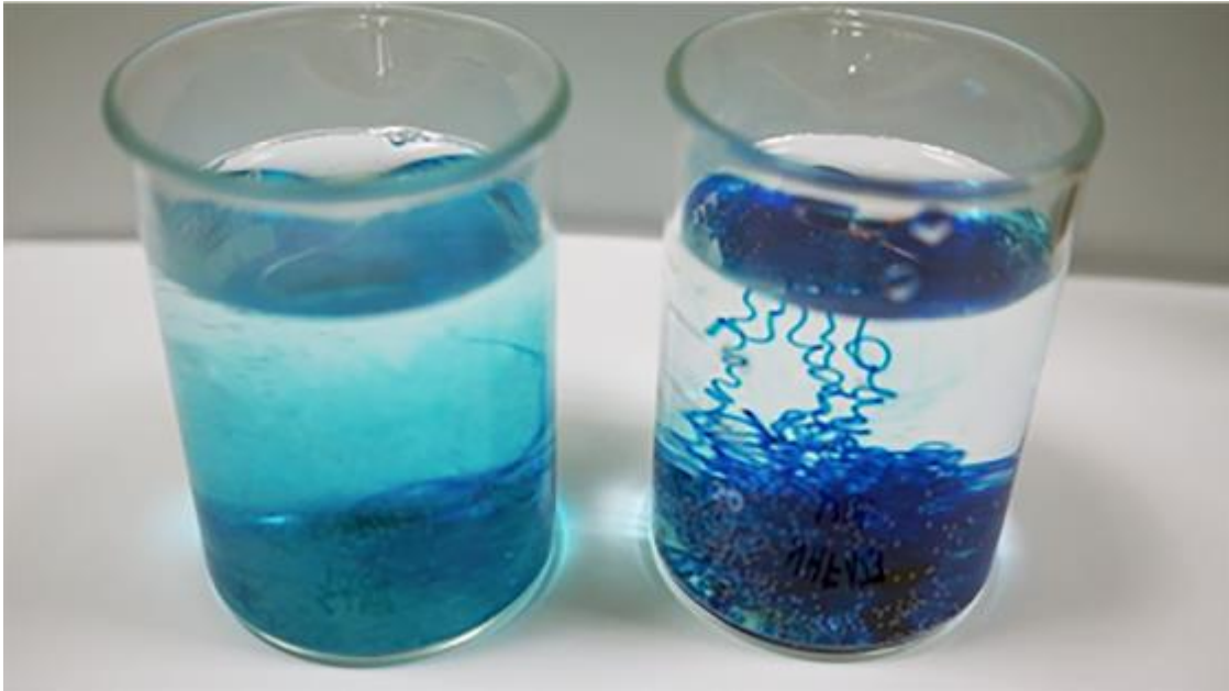
Figure 14. Image of injected P407 (left) and NHP407 (right) solutions with 20%w/v concentration (prepared and conditioned at 5°C) in a water bath kept at 37 °C. NHP407 hydrogel rapidly forms after injection and assumes a fibrous shape, while P407 hydrogel with the same concentration shows the tendency to rapidly dissolve in contact with water.
