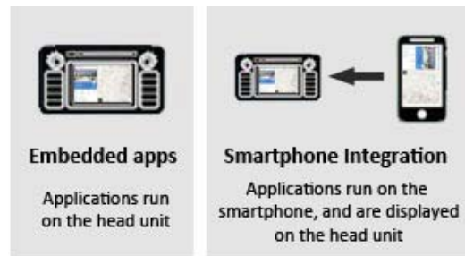
Fig. 6. Two alternatives for providing infotainment applications.
