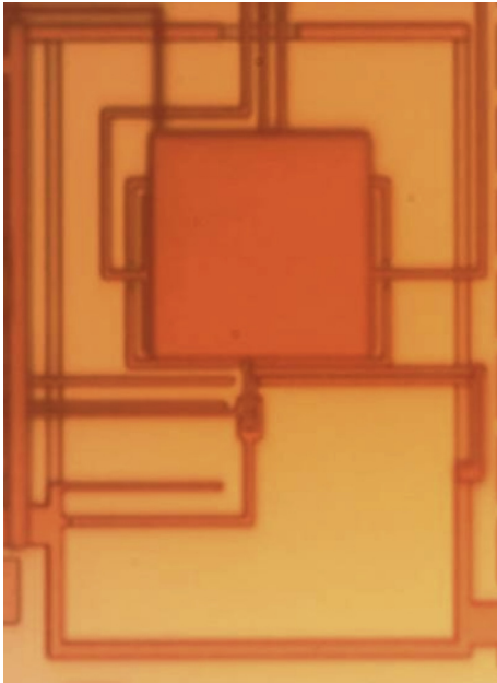
Fig. 3. Microphotographs of a radiation sensor with metal 3 shield ('M3' sensor) over the FG. The shield is accessible via external pads to allow high voltage bias to be applied to it.
