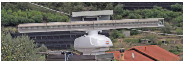
Figure 3. Harmonic radar for the yellow-legged hornet tracking. The TX antenna is 180 cm long, while the RX antenna (on top of it) is 50 cm long.
