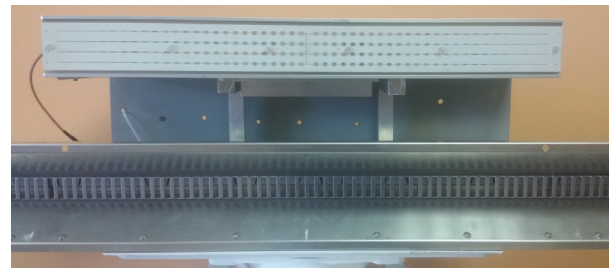
Figure 8. Receiving antenna (50 cm long) designed realized in microstrip on top of a portion of the transmitting slotted waveguide antenna.
