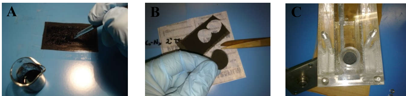
Figure 20. Pictures of the Gas Diffusion Electrode preparation: catalyst ink deposition on the GDL (A), GDL disk cutting (B) and positioning in the holder of the plexiglass cell (C).
