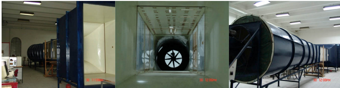
Figure A.1: Wind tunnel air inlet.
