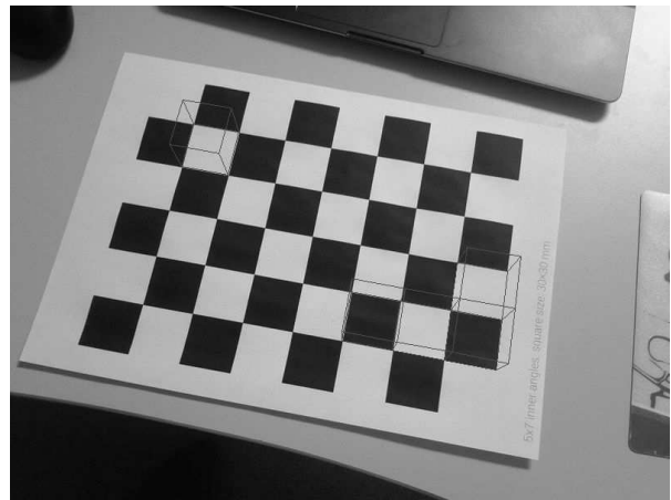
Fig. 6. The camera calibration. To check the quality of the calibration some virtual 3D blocks are displayed on the calibration chessboard.
