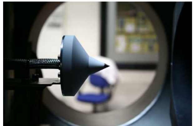
Figure 6: Double cone probe installed in the test chamber.
