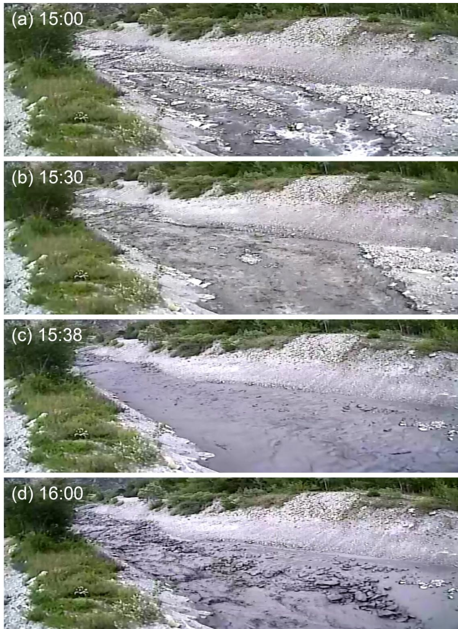
Figure 23 - Frames of the video recorded on July 17, 2013 by the video camera located along the road (see plan in Figure 18). In the first frame, the torrent in steady regime (h 15:00); in the second one the first surge (h 15:30); in the third frame, the mud flow front (15:38); in the last one, the tide (h 16:00).
