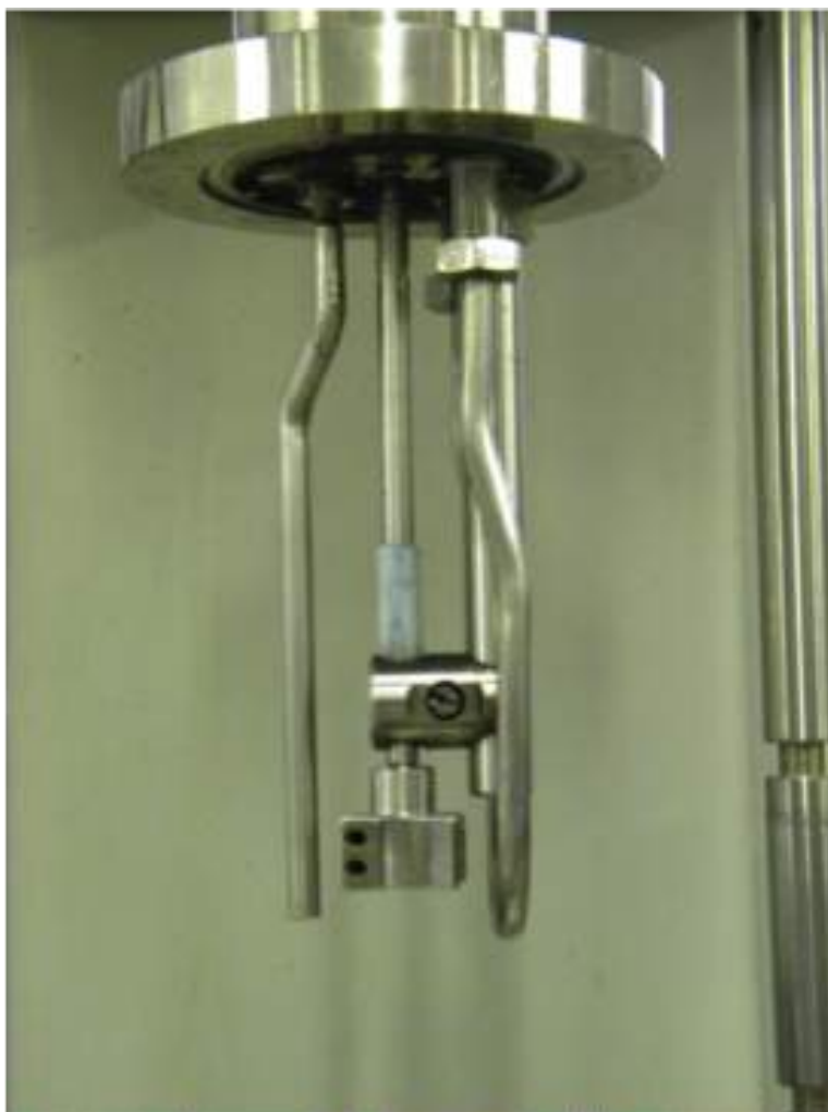
Figure 6.3: The interior of the reactor; it is possible to observe the holed impeller, the cooling loop on the right side and the pipe for the gas injection
