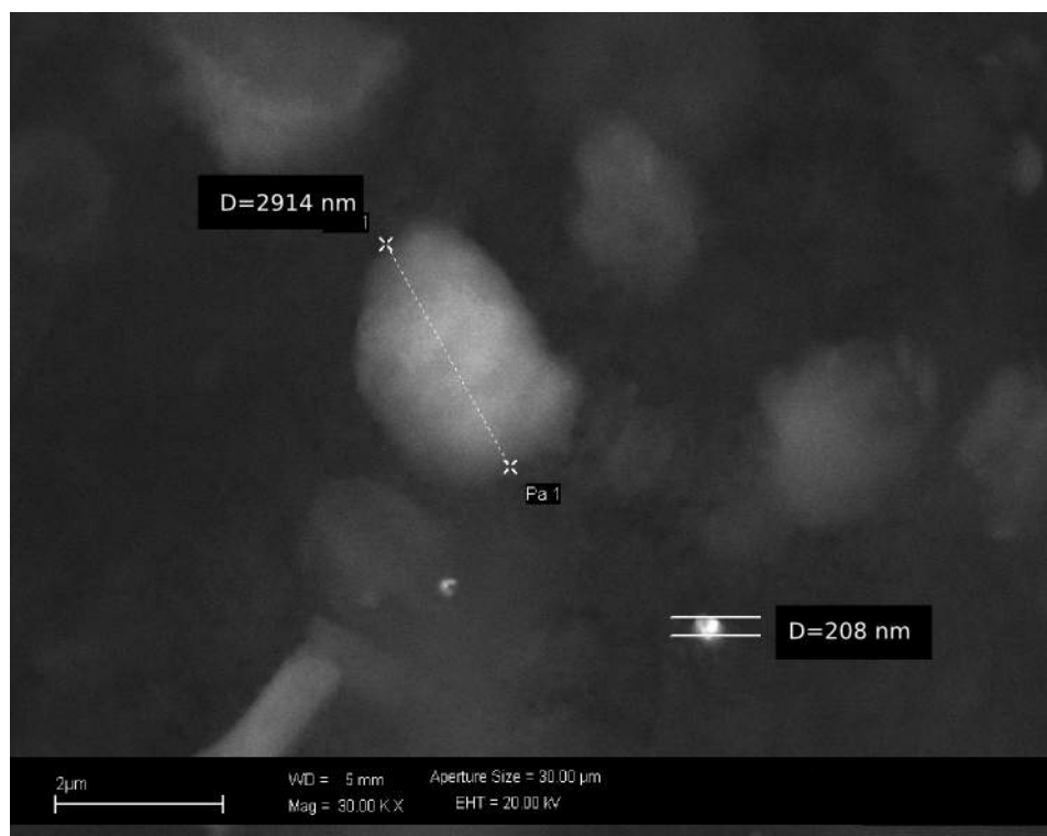
Figure 4.21: The FESEM image takes from the sample with Au NPs synthesized with impregnation method; support: carbon black
