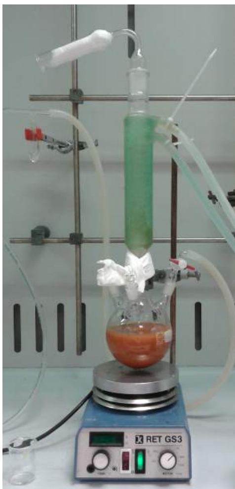
Figure 4.6: An example of the reactor for the complex synthesis in its monomeric form
