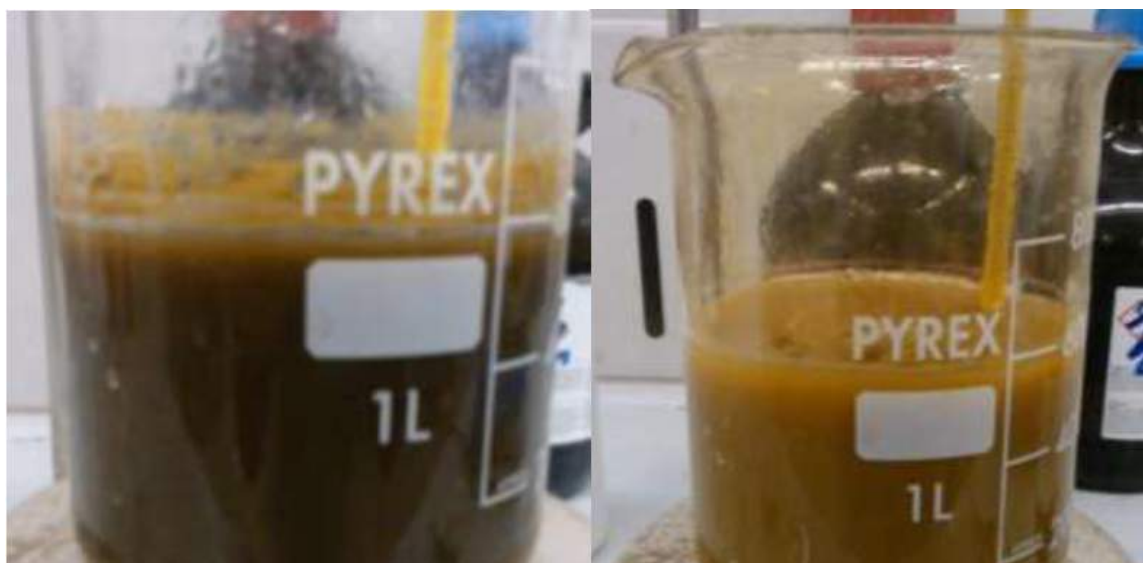
Figure 8.1: This picture was taken during the reaction and 2 hours mixing (after water addition at 98°C)
