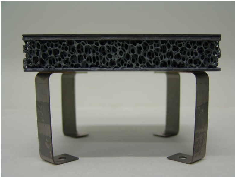
Figure 7.9 150x150 mm 2 technology sample
