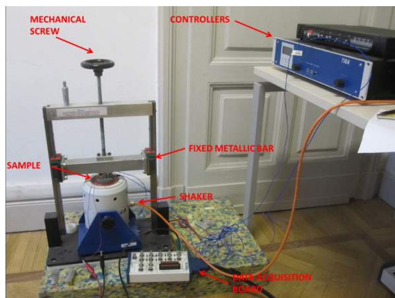
Figure 5.17. Image of the whole set-up for the piezoelectric output voltage generation measurements, including the mechanical shaker, the controllers, the data acquisition board and the fixed structure for compression measurements.
