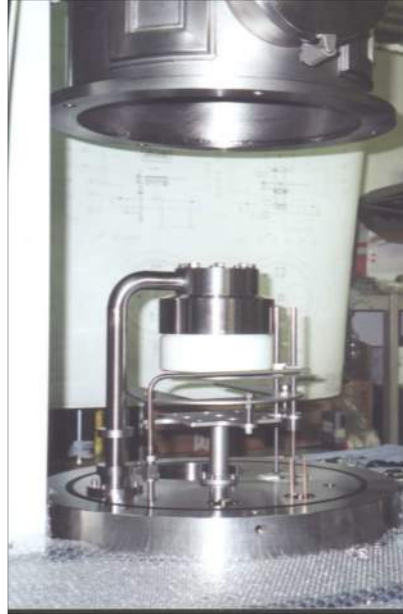
Figure 3.3. RF magnetron sputtering monotarget system - View of the inner part of the deposition chamber.
