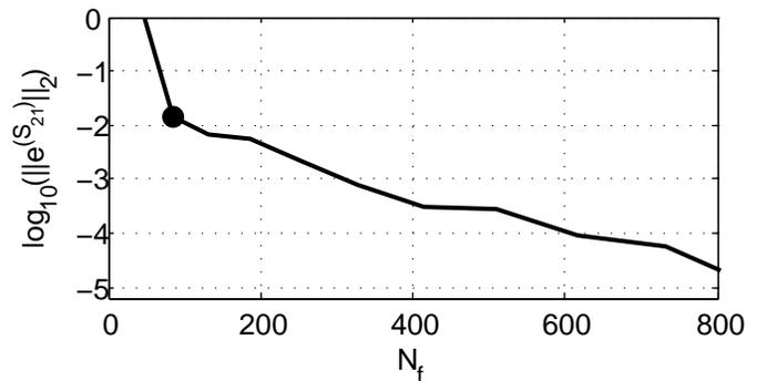
Fig. 8. Convergence analysis of the MEM applied to the array of dielectric rods of Fig. 3. The curves report the 2-norm relative error  $\|e^{(S_{21})}\|_2$  in the transmission coefficient versus the number of functions used to represent each unknown of the differential problem. The dot refers to the simulations of Fig. 6.
