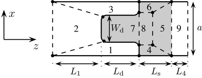
Fig. 9. Domain decomposition approach applied to the realistic model of a surface-relief diffraction grating. The patches 4 ÷ 8 are filled with dielectric  $\epsilon_r = n^2$ , the remaining ones with vacuum; the dots identify the vertices of the patches; all the corners are rounded, with radius of curvature  $R$ .
