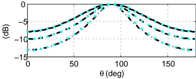
Fig. 5. Magnitude of the  $TE_0$ - $TE_0$  mode reflection coefficient for the array of dielectric rods of Fig. 3, with  $R = L_d/40$ ,  $f = 1.2$  THz. The solid, dashed and dash-dotted lines refer to results obtained with  $\varphi = 20^\circ, 40^\circ, 60^\circ$  with the MEM technique. The brighter, dotted lines refer to the results obtained with MoM.
