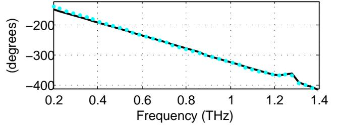
Fig. 11. Magnitude and phase of the  $TM_0$ - $TM_0$  reflection coefficient for the surface-relief diffraction grating of Fig. 9, with  $R = L_d/4$ . The solid and dotted curves refer to results obtained with the MEM technique and with CST-MS, respectively.
