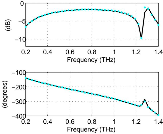
Fig. 10. Magnitude and phase of the  $TE_0$ - $TE_0$  reflection coefficient for the surface-relief diffraction grating of Fig. 9, with  $R = L_d/4$ . The solid and dotted curves refer to results obtained with the MEM technique and with CST-MS, respectively.
