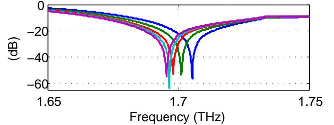
Fig. 7. Magnitude of the  $TE_0$ - $TE_0$  mode reflection coefficient for the array of dielectric rods of Fig. 3. The curves from right to left refer to  $R = L_d/3, R = L_d/4, R = L_d/6, R = L_d/9, R = L_d/40$ .
