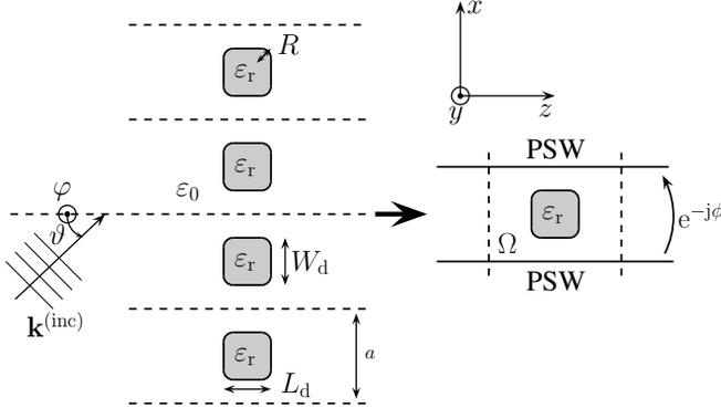
Fig. 1. Left: sketch of the geometry of the structure; right: unit cell. The horizontal solid lines are phase-shift walls (PSW) with phase shift  $\phi = k_x^{(\text{inc})} a$ ; the vertical dashed lines define the access ports; the parameter  $a$  is the period;  $L_d$  and  $W_d$  are the dimensions of the dielectric rod;  $R$  is the radius of curvature of the rounded corners.
