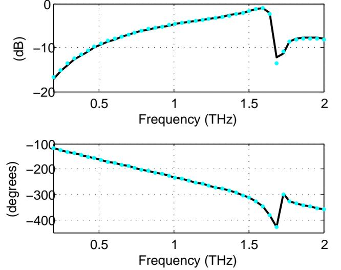
Fig. 6. Magnitude and phase of the  $TE_0$ - $TE_0$  mode reflection coefficient for the array of dielectric rods of Fig. 3, with  $R = L_d/4$ . The solid and dotted curves refer to results obtained with the MEM technique and with CST-MS, respectively.
