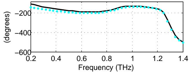
Fig. 12. Magnitude and phase of the  $TM_0$ - $TE_0$  ( $TE_0$  incident) reflection coefficient for the surface-relief diffraction grating of Fig. 9, with  $R = L_d/4$ . The solid and dotted curves refer to results obtained with the MEM technique and with CST-MS.
