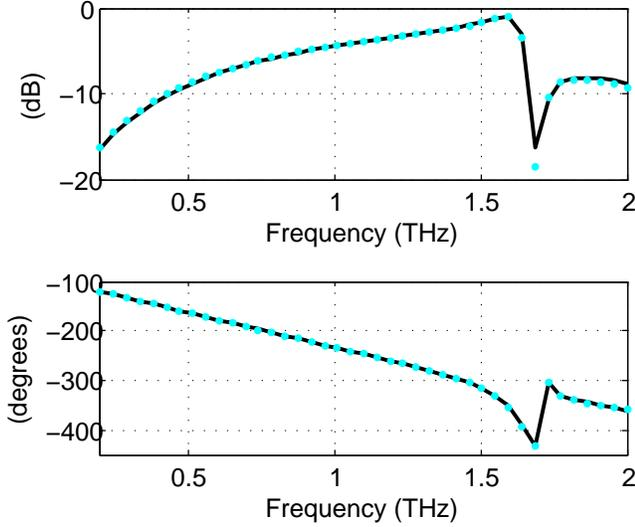
Fig. 4. Magnitude and phase of the  $TE_0$  mode reflection coefficient of the array of dielectric rods of Fig. 3, with  $R = L_d/40$ . The solid and dotted curves refer to the MEM and with MoM simulations.
