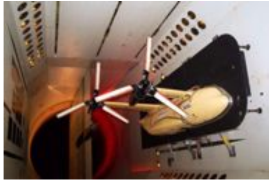
Figure 1.6: Boeing Quad Tilt-rotor Half-model in the Langley Wind Tunnel
