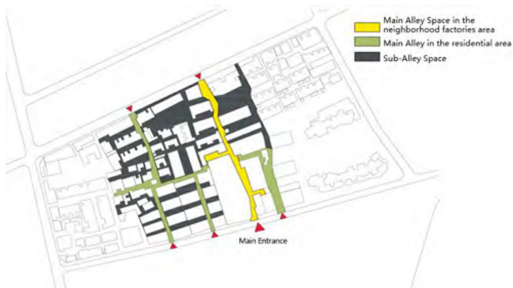
Figure 5-20 Analysis of alley space in 2008 (Source: edited by author. According to GUO Chunbin, “Research on the Spontaneous Rehabilitation of Old Residential Areas,” in Urban planning conference 2011 , 2011, pp. 7413–7425.)
