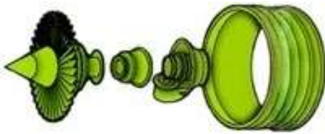
Figure 15: Exploded view of the fan major module of the CFM56-7 engines [26]
