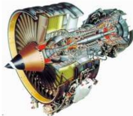
Figure 12: Schematic cutaway representation of CFM56-7B developed by CFM International
