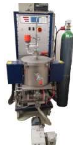
Figure 108: GERO furnace for heat treatment of \gamma -TiAl alloys
