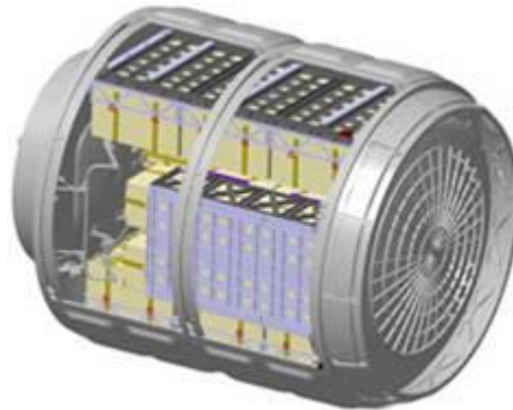
Figure 67 CLV pressurized payload configuration, ref. [42]
