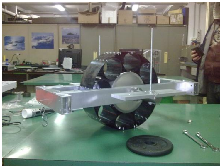
Figure 96 A structural similitude model: the “scaled wheel”
